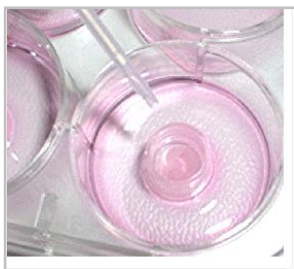
Figure 5: Application of semisolids (positive displacement pipette - detail)
